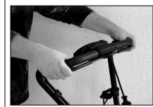
Pull the lower lever: \* Rotary brush drive ON
